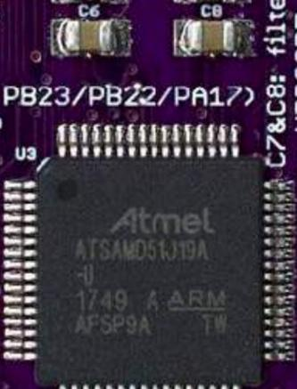
C7&C8: filter caps on VDDCORE, output from the chip's voltage regulator.
