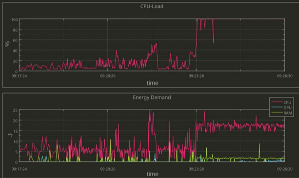
Figure : Monitoring energy and hardware consumption in real time with KDE's LabPlot (image published under a CC-BY-NC-ND-4.0 license).
