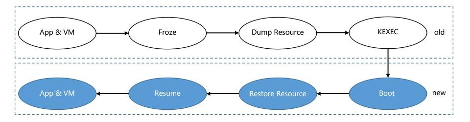
\* time cost = dumping time + kernel switch time(KEXEC) + restoration time
