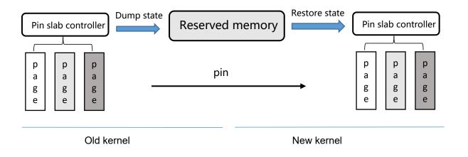
\* Create a pin slab controller to manage the old kernel pages which need to keep constant while booting the new kernel.
