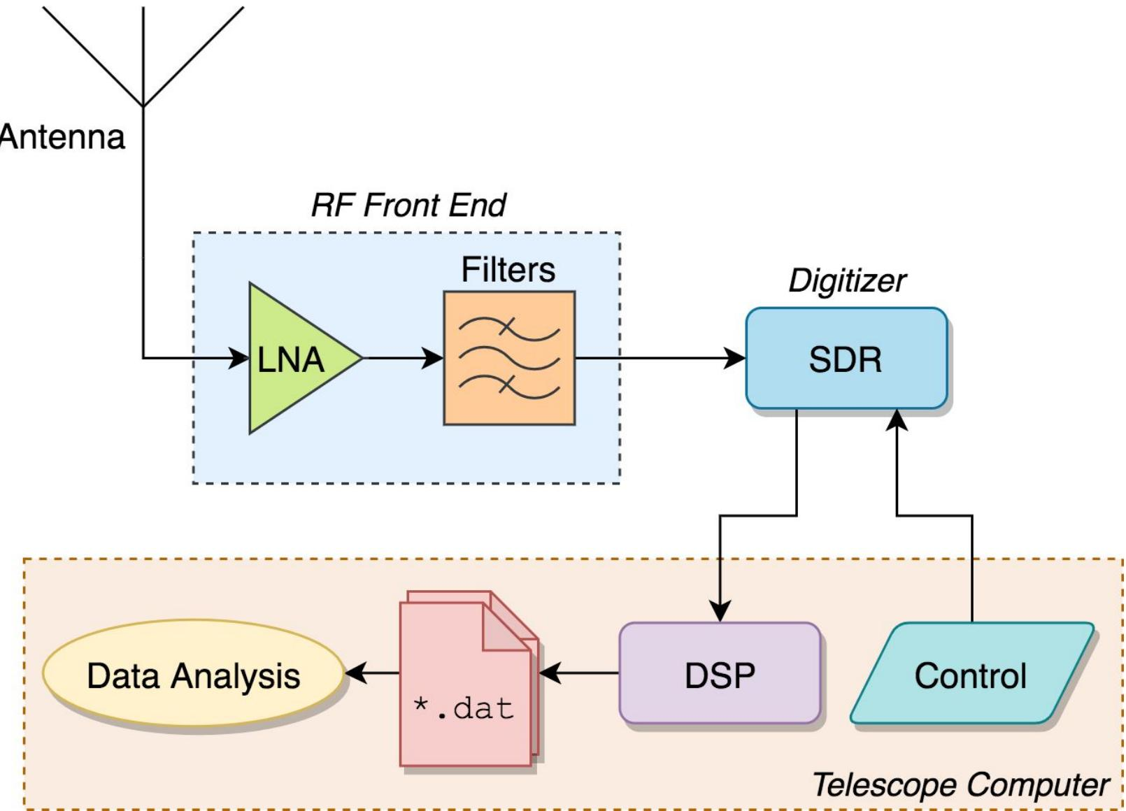
Fig. 1: Typical block diagram of a Radio Telescope.
