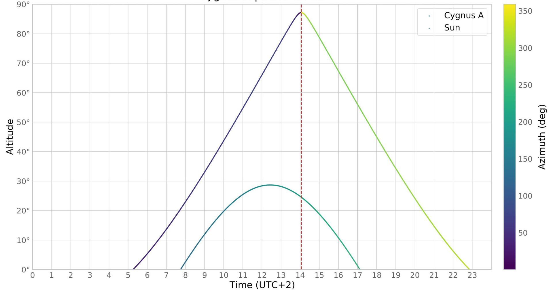
**Fig. 5:** Example prediction of the location of the Cygnus A radio galaxy (3C 405) in the celestial sphere of the observer.
