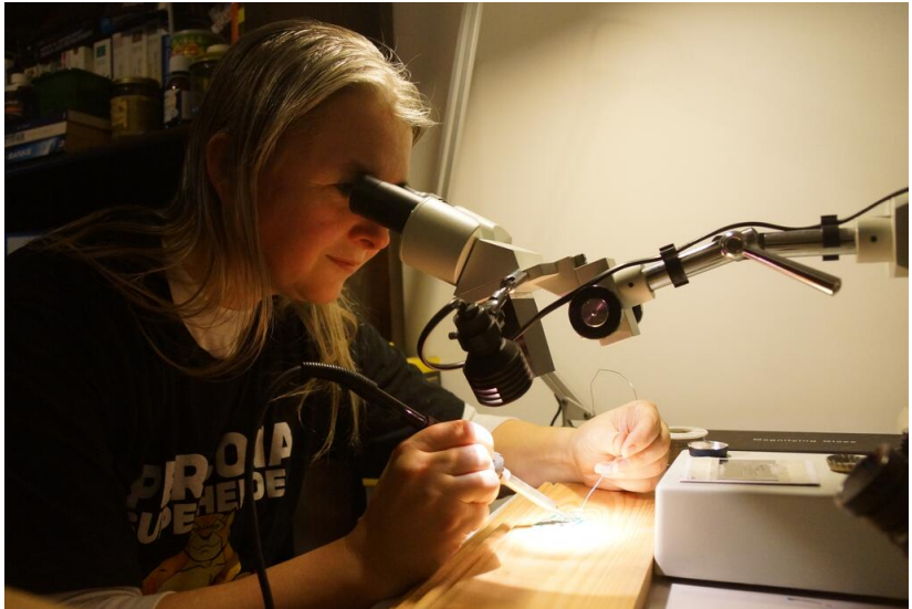
Figure 17: using a microscope for soldering
