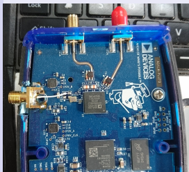
Externally clocked ADI PlutoSDR
