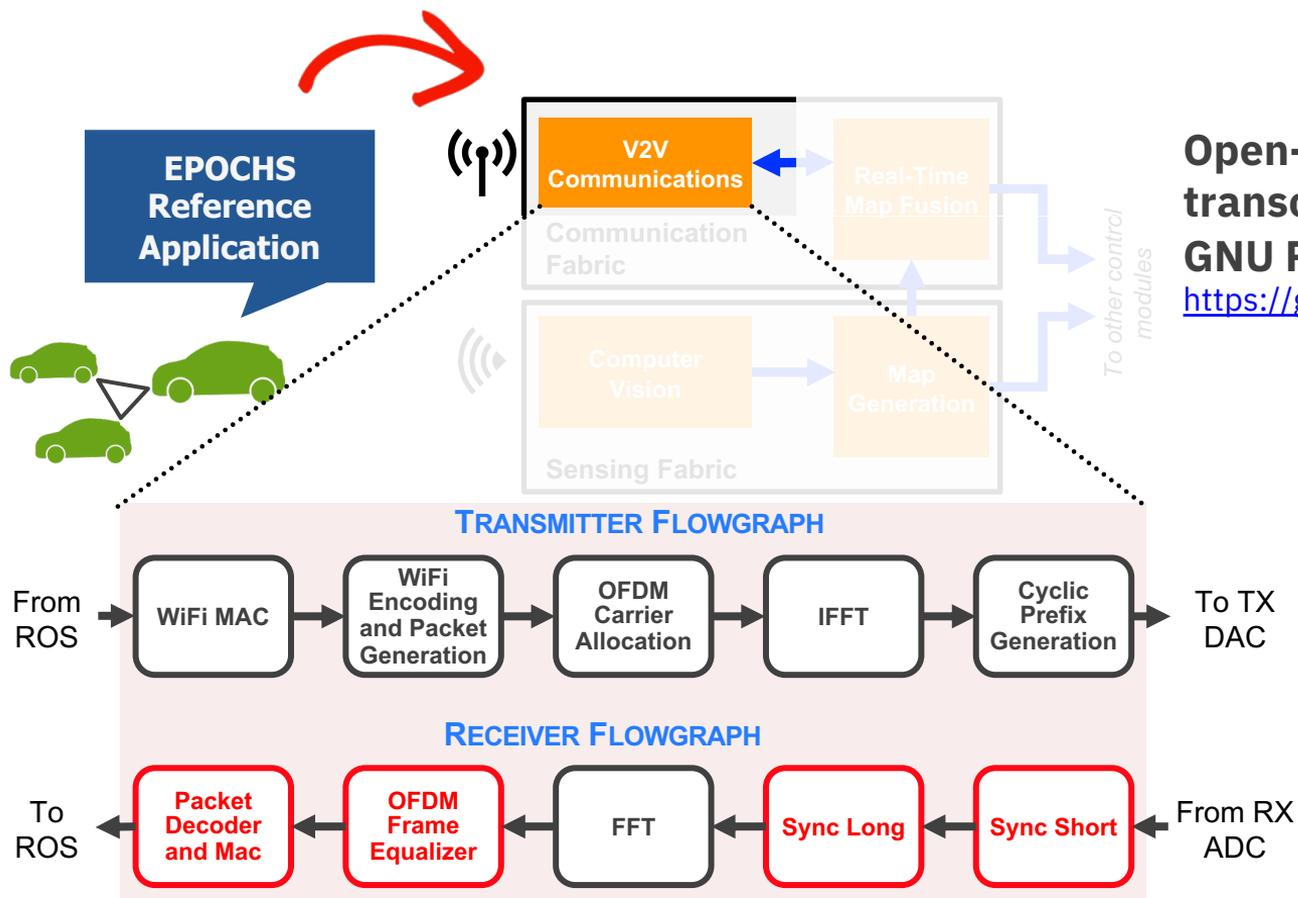
Open-source IEEE 802.11p transceiver implemented in GNU Radio by Bastian Bloessel
