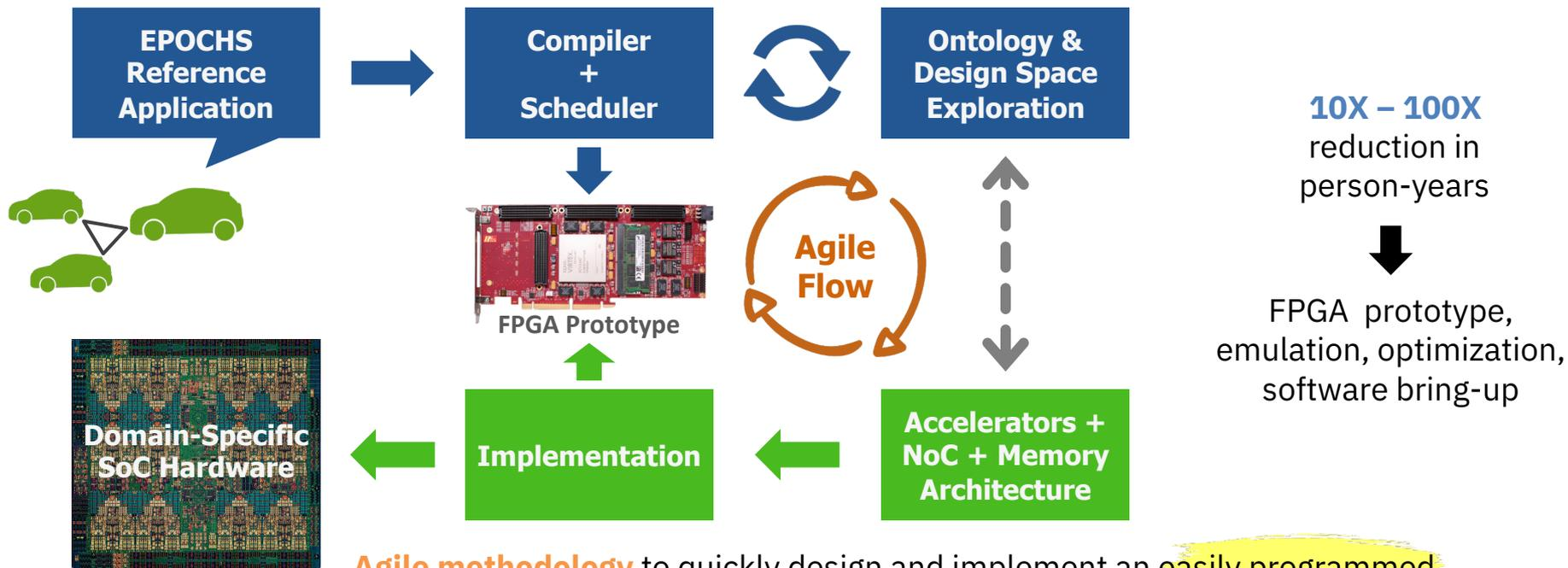
**Agile methodology** to quickly design and implement an **easily programmed** domain-specific SoC for real-time cognitive decision engines in connected vehicles
