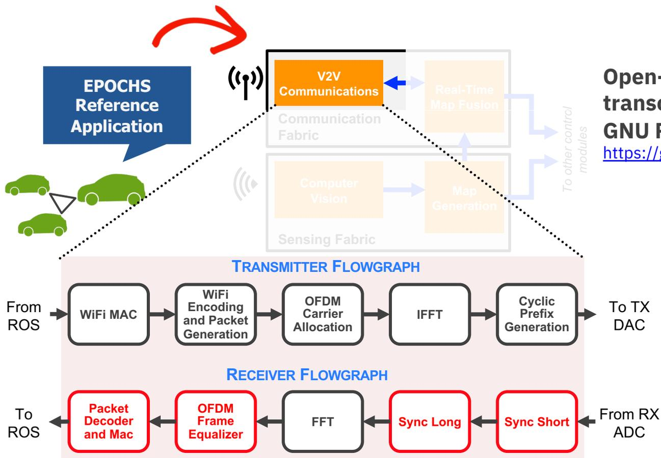
Open-source IEEE 802.11p transceiver implemented in GNU Radio by Bastian Bloessl
