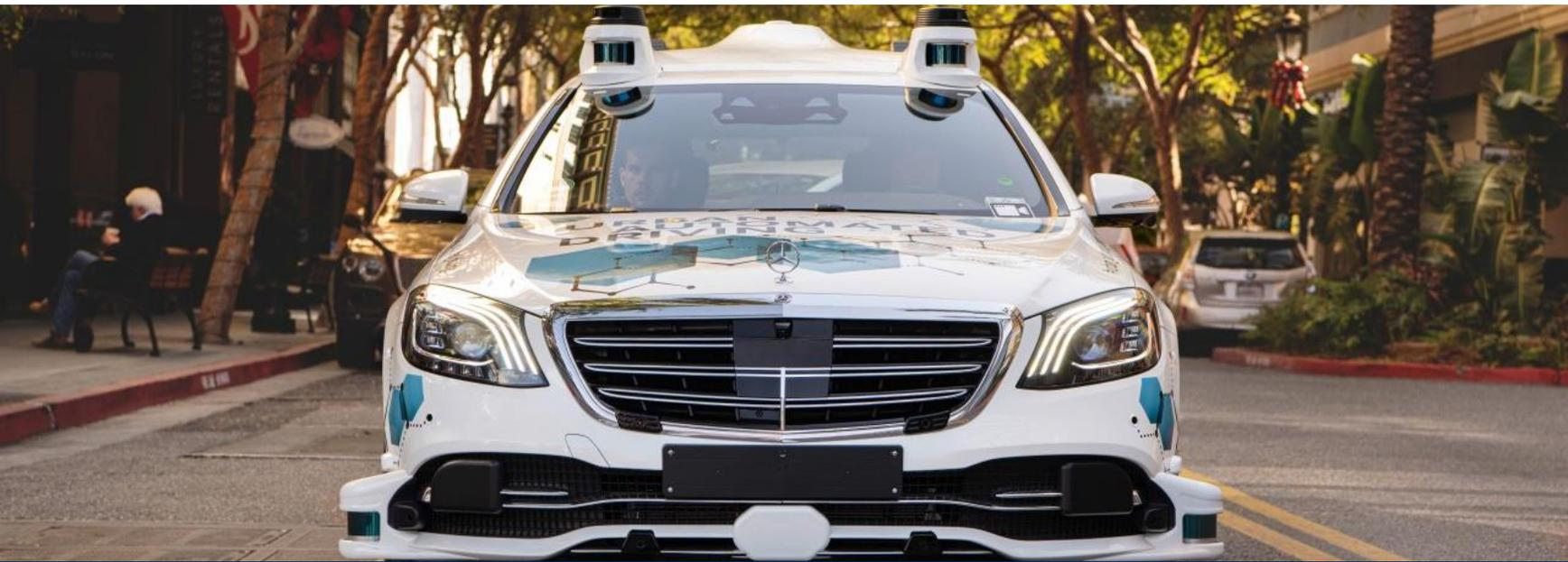
automated driving is a data processing chain with sensor input of up to 10 GB/s
