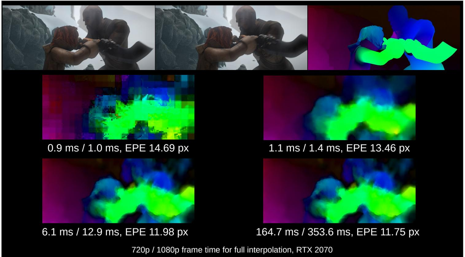
So, how good is our estimated flow? This is a test sequence from the so-called MPI-Sintel benchmark (using Sintel from the Blender Foundation). Since it's synthetically rendered, we have exact motion vectors for every pixel, and can compute the endpoint error (EPE) over the entire 50 frames.
