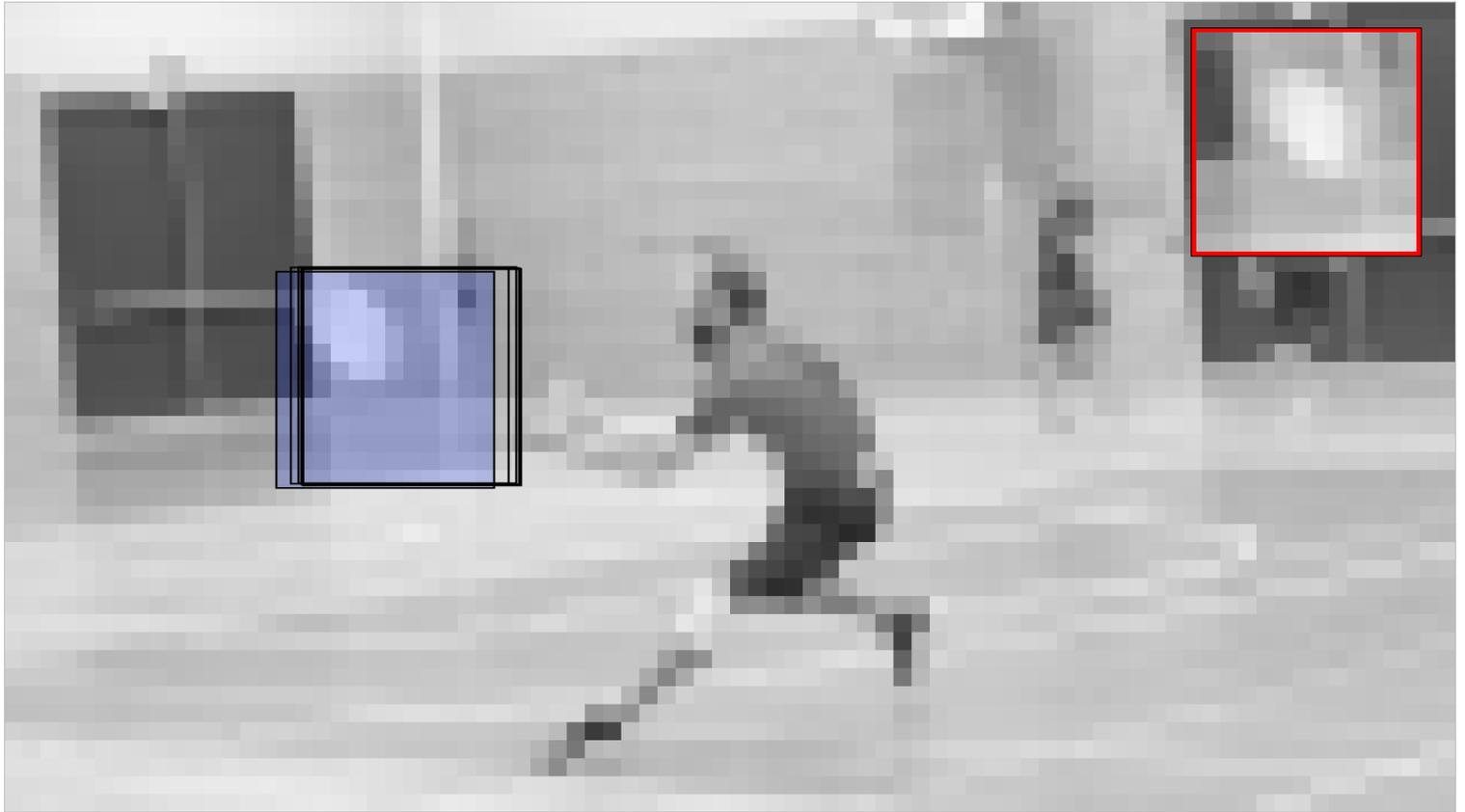
Let's go through the algorithm on a high level. We start with a motion search on low resolution; divide up the image in a series of overlapping blocks, and search for a similar block in the other image.
