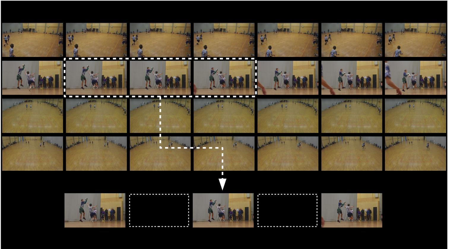
Enter Futatabi. It works as a multi-track recorder—everything is recorded, all the time. It gets the frames from Nageru over a standard network; I've chosen MJPEG as the codec, as it's reasonably high-quality and has hardware encoders/decoders in recent Intel GPUs. We have roughly 75 Mbit/sec/camera in 720p, or 125 GB/hour for four cameras.
