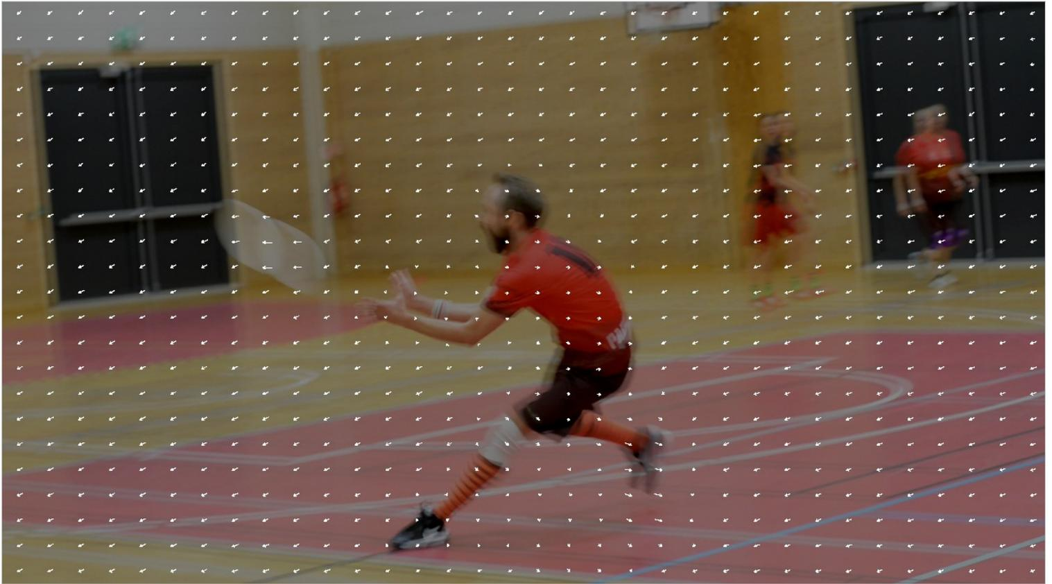
So once we have a flow field between the two frames, we can halve and then somehow invert it. (We won't be discussing this step in detail—it's a bit trickier than it looks at first sight.) This would give us, for the intermediate frame, where to fetch each pixel *from*, which is more directly useful than where it wants to *go*.
