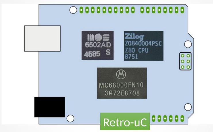
micro-controller with Z80, MOS6502, Motorola 68000 cores Tomorrow Talk @ Retrocomputing Devroom: Retro-uC
