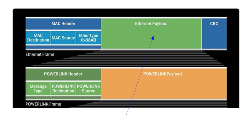
Powerlink frame "inside" Ethernet payload
