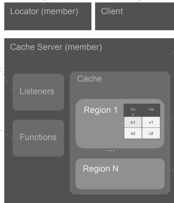
CacheServer - process connected to the distributed system with created Cache
