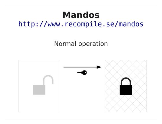
An unlocked and running server provides the password needed by a locked server when the latter boots.
