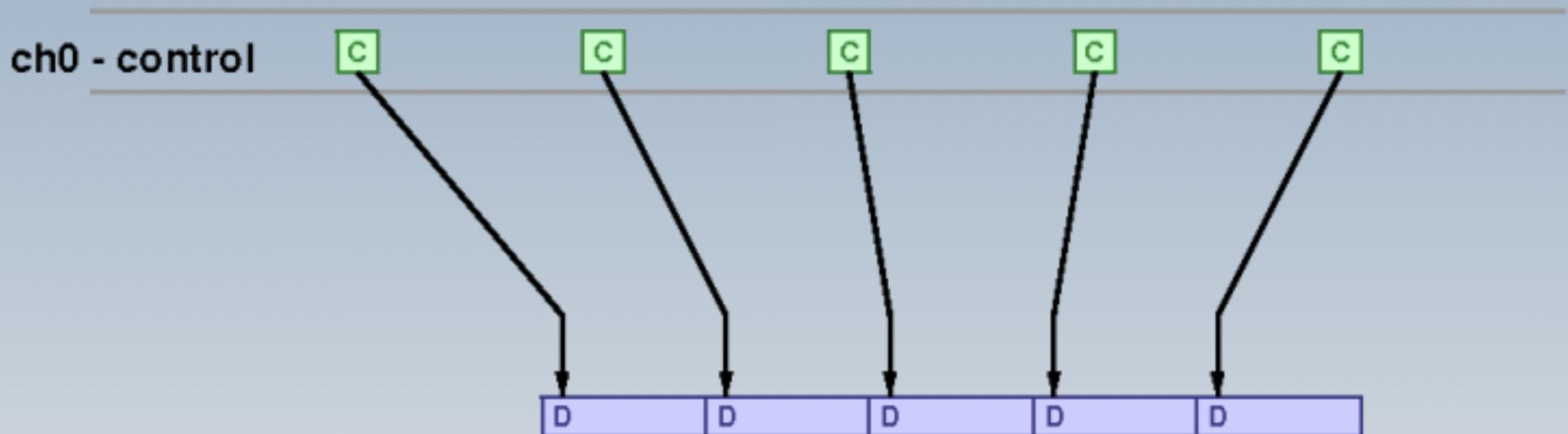
The control channel times I/O and refers to mmap data
